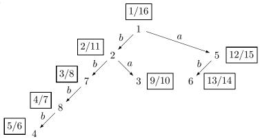
Notation E/F is used, whereas E indicates the step number at the entering into the current state ("enter") and F the step number while leaving the current state ("farewell"). Edge-reversed Automaton  $\overline{\mathcal{A}}$ :
